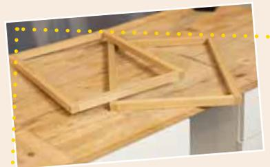
Drill holes into the ends of the boards and connect them to form two identical frames using the screws. Paint the frames if desired.
