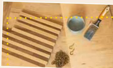
First saw the boards into uniformly sized pieces: Four of the pieces should be as long as the short side of the board. The other four pieces can be a little bit longer.
